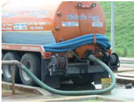
The Indian River County Residuals Dewatering Facility receives large volumes of septage, about 378,500 L/d (100,000 gal/d), from 30 to 35 vacuum trucks. Indian River County and Lakeside Equipment Corp.
